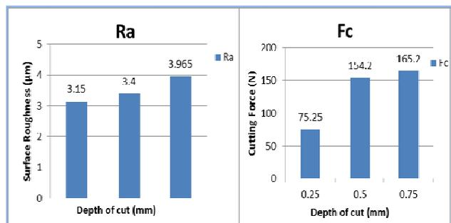
Fig. 6: Influence of depth of cut on surface roughness and cutting force
