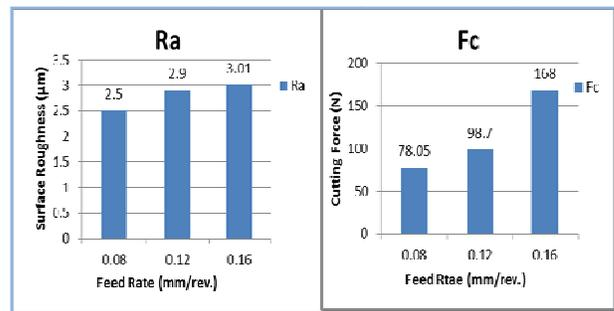
Fig. 5: Influence of feed on surface roughness and cutting force
