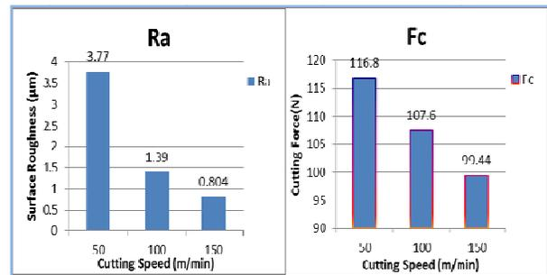
Fig. 4: Influence of cutting speed on surface roughness and cutting force
